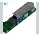
All sensors and options (second control unit, photoelectric ceiling barrier) with electric supply can be plugged into circuit board (plug 'n' play).
