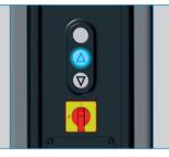
Lower end position reached or an obstacle has been hit. Only lifting is possible. Raise button lights up blue.
