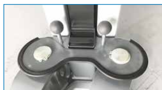
Protection stop for vehicles with low doors (MA STAR 3.5 A/S).
