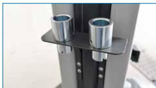
Sheet metal tray for support disc extensions.
