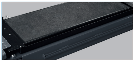
Slide plates with 60 mm transverse adjustment range and 5 ° turning range (optional)
