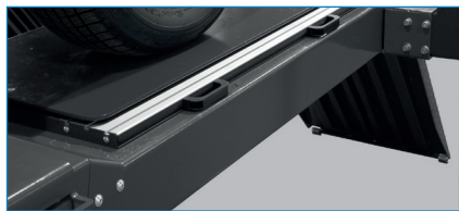
Precision slide plate (optional, available only for version "W"): Very small breakaway torque of 5 Nm and very small slide force of 15 N required at 500 kg wheel load, large amount of steel balls, hardened running surface, collector channels for dirty water (Right-hand picture: upper plate removed)
