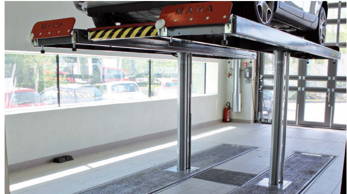
Vehicle lifted by the wheels
