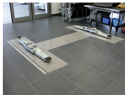
With closed covers, the lift can be used as a standard lift
