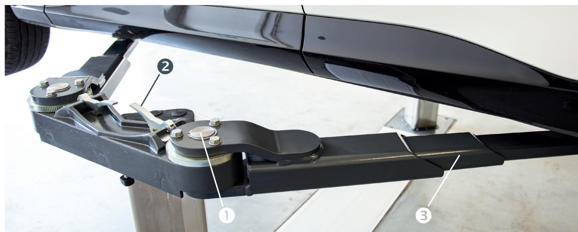
Swing arm support with tool tray.
