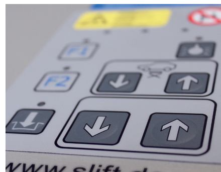
Membrane keypad with easy-to-operate micro-switches
