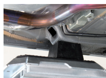
Pyramid block for highly accurate support and high freedom of movement underneath the vehicle.
