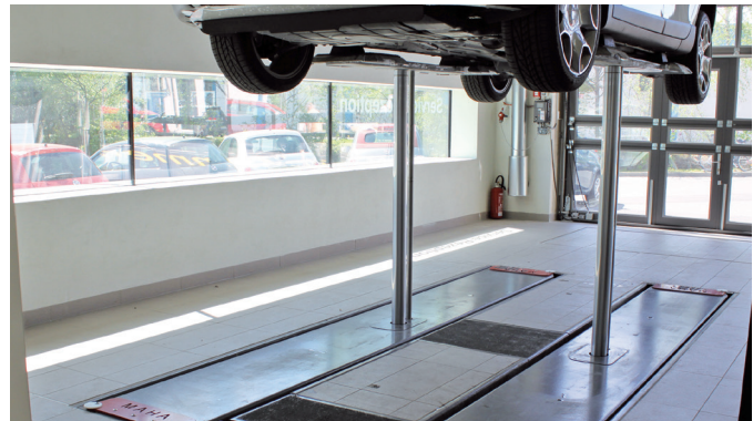
Vehicle lifted by the sill
