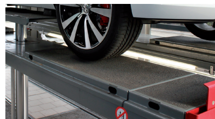
Runways with compensating plates for level adjustment to wheel-free jack or wheel alignment.
