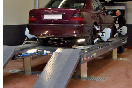
Highly accurate as a wheel alignment lift
