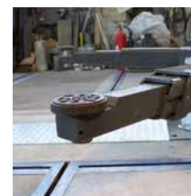
101 mm minimum height of support disc
