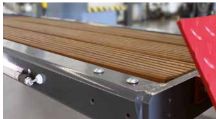
Runways with wooden coverage for durable wheel tread and cutting edge design.
