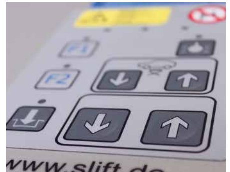
Membrane keypad with easy-to-operate micro-switches
