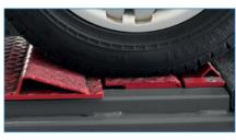
Rear prism half is automatically lowered, all four wheel contact surfaces are level.
