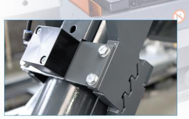
The toothing of the mechanical locks for wheel alignment lifts is machined by milling (option "Lowering Device"). This ensures high measuring accuracy at different working heights.
