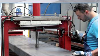
Option "Lowering Device": After welding, the runways for wheel alignment lifts are straightened exactly flat in the area of the turntables and sliding plates.
