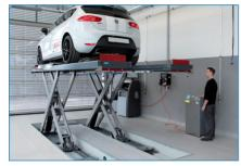
Effective height of min. 1850\*\* mm with installation in strip foundation.
