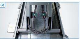
Cables and hydraulic hoses placed within the scissors tubes and in energy guidance chains. Optimum protection against damage! With the generous lifting height of ca. 2100 mm ideal for installation in a strip foundation or in conjunction with a centre platform.
