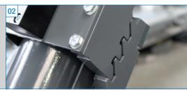
The pneumatically activated latch serves as a safety against downward movement with hydraulic leakage.
