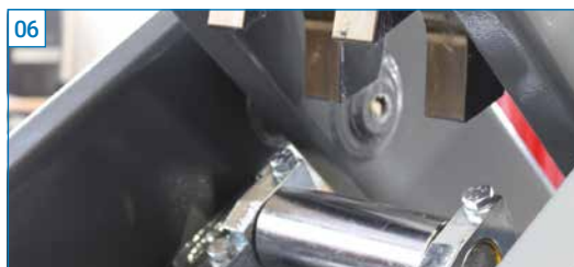
The cylinder raising support with step lever and rollers conducts a pure rolling movement. No sliding movement between the moving parts, meaning it is low noise, wear resistant and nearly maintenance-free.
