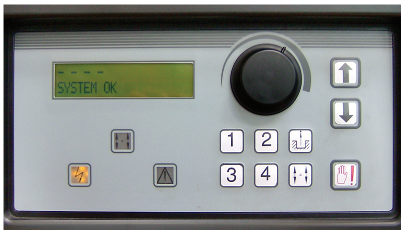
Standard delivery with electronic synchronization control of the complete lifting system with approval based on DIN EN 1493.
