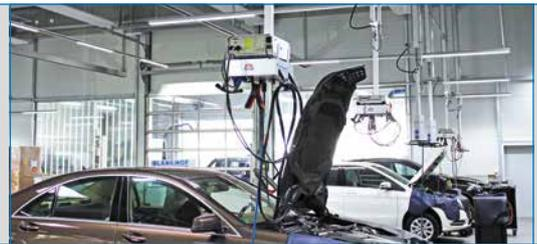
Installation examples of MAHA media supply during workshop operation. The E-BOX versions are individually adjustable to each workstation and ensure ergonomic working.
