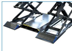
The lift can be moved using a conventional dolly or forklift thanks to the optional mobile frames. The lift requires no anchoring to the floor, the installation frame is self-supporting and only requires a solid ground surface. The drive-over height of the lift is increased by only 12 mm (TWIN F IV 3.5 A).
