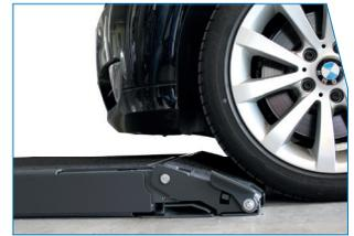
With a drive-on height of no more than 105 mm, the hinged extensions also serve as access ramps.
