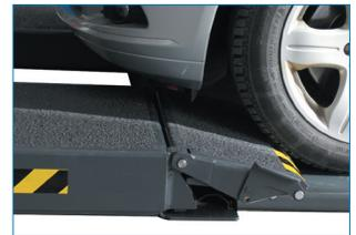
... reduce the drive-over height to 65 mm, which allows easy access to the lift even for vehicles with very low ground clearance.
