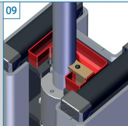
Straightforward lubrication of the spindle as container filled with oil.
