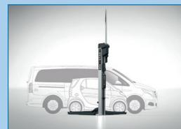
Can hold vehicles from mini-cars to vans (e.g. SMART fortwo and VW T6 long 3.5 t resp. up to MB Sprinter and VW Crafter long wheelbase 5.5/6.5 t).
