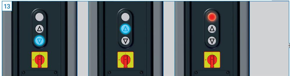
Upper end position or photoelectric ceiling barrier reached. Only lowering is possible. Lower button lights up blue.
