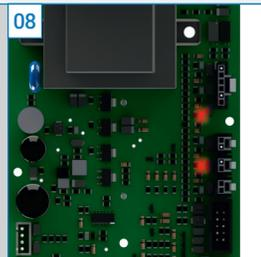
Simple visual error diagnostics thanks to LEDs mounted on the circuit board.
