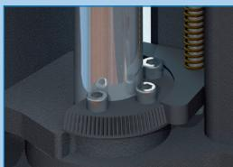
Maximum safety thanks to arched support-arm restraint with operation across the entire length with small ratchet graduation.
