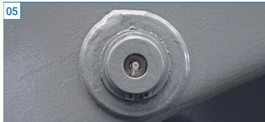
Scissors main bearing with Teflon bearing bushing and
