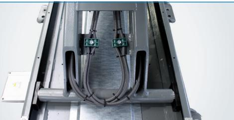
Cables and hydraulic hoses placed within the scissors tubes and in energy guidance chains. Optimum protection against damage!
