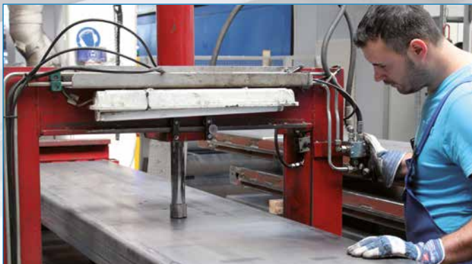
Option "Lowering Device": After welding, the runways for wheel alignment lifts are straightened exactly flat in the area of the turntables and sliding plates.
