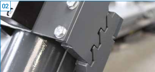
The pneumatically activated latch serves as a safety against downward movement with hydraulic leakage.
