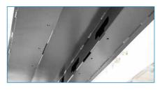
Additional reinforcement plates within the runways welded for high torsional and bending stiffness.
